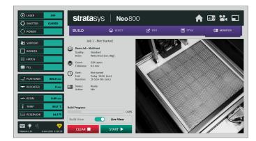
Each Stratasys Neo system is installed with a built-in camera, allowing users to keep track of builds remotely, at any stage.
