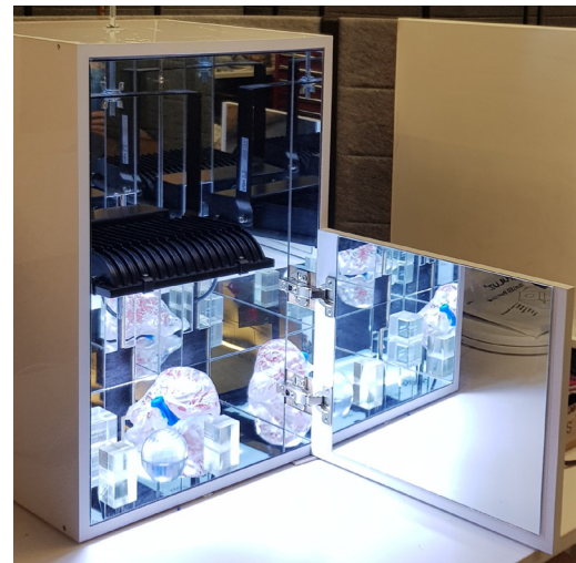
Figure 5: Sample do-it-yourself photobleaching cabinet with LED lamp and mirrors
