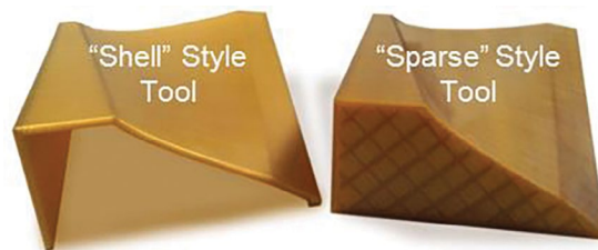
Figure 2 – FDM tool construction styles.
