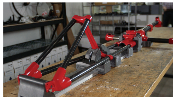
Figure 7: Utah Trikes uses FDM Nylon 12CF material in its advanced prototyping.
