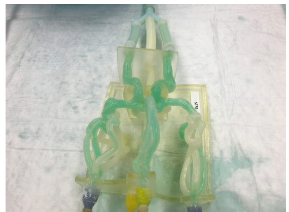
Figure 6: The Jacobs Institute 3D prints vascular models using Agilus30 material and PolyJet technology.
