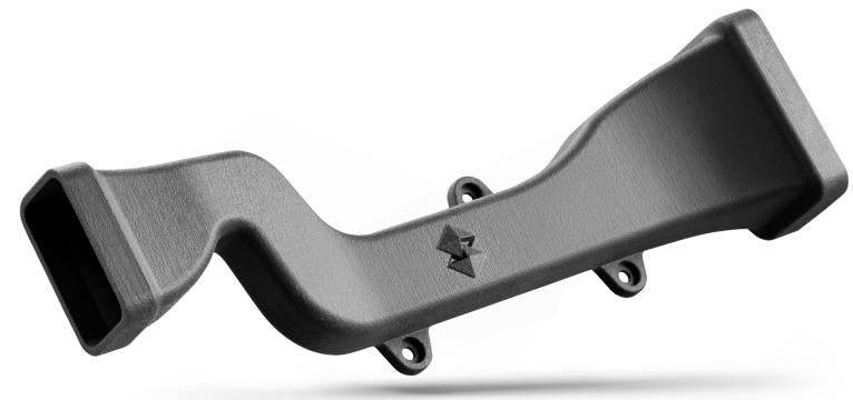
This air duct part of an automotive HVAC system, printed with SAF<sup>™</sup> technology. Traditionally, a part like this might be molded as two halves and assembled. With SAF technology, the halves can be produced as a single part, reducing post process assembly and points of failure.
