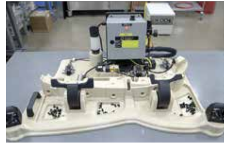
Automotive assembly jig built in ULTEM™ 9085 and FDM Nylon 12™ material.
