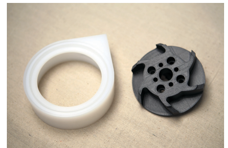
The 3D printed impeller prototype (black) works with its PC mate to push an ice slurry through a chilling system.
