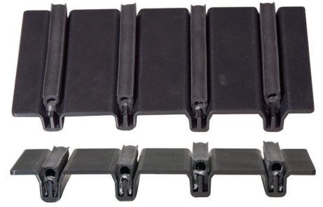
This FDM part (top and side view) allows testing of four variations of a groove that mates with a rubber seal. The finished HVAC system housing (below) features three FDM parts.
