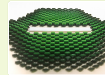
Heel spur graphics 3D Printed directly onto fabric substrate
