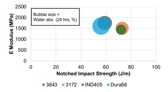
Origin has a robust portfolio of tough materials featuring different colors, performance profiles, and cost points. The three materials shown above are good choices for parts and applications in high impact environments (manufacturing jigs) or frequently opened and closed (latches).
