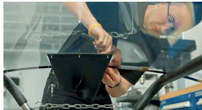
Tim Murphy, part designer, installs air flow duct onto Next Gen car windshield.
