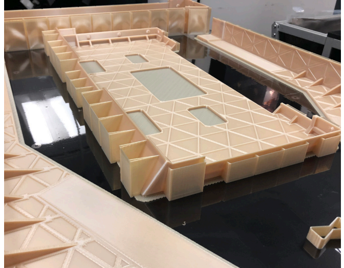
These 3D printed parts replace assemblies that were previously made using a more resource-intensive composite laminate process.
